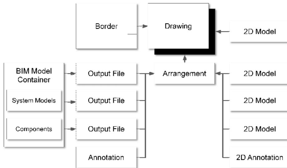
*In the diagram above, the Output files are created from the BIM model to allow integration with the 2D CAD system. The drawing is then compiled in the 2D CAD system so that all designers have access to view and print the drawings, even if they do not have the BIM software installed.*
