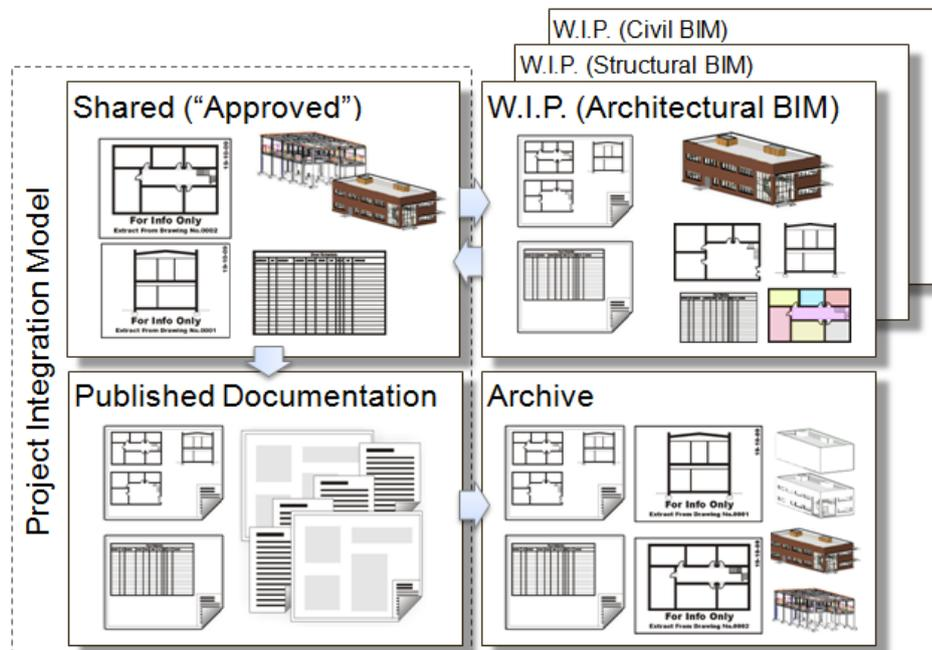
Information for each discipline is created in their own Work In Progress (WIP) area. This is typically located on the data (or projects) server within each company's own unique Local Area Network. No-one has access to any BIM data in the WIP areas apart from the content owner.
