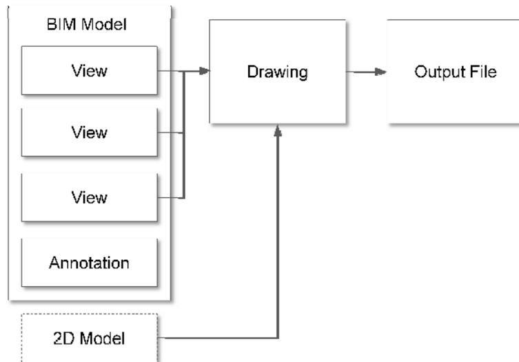
*In the 100% BIM Workflow diagram, all views and annotation are created from within the BIM system. Additional 2D references may be attached as required. Output files are then exported from the drawing sheet for integration with 2D CAD systems or issue to external parties.*
