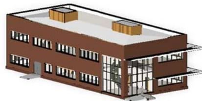
Concept components substituted for Grade 2 or 3 components as design progresses.
