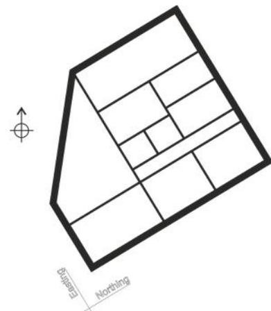
Data exported from the BIM can then be either real world or local and whilst the majority of data will need to be delivered in OS co-ordinates for the purposes of collaboration and cross-referencing, some software (e.g. certain structural analysis software) requires data to be located at 0,0. For export to such software, local coordinate systems can be utilised.
